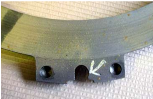
Reclaim tang slots and reaction face.
