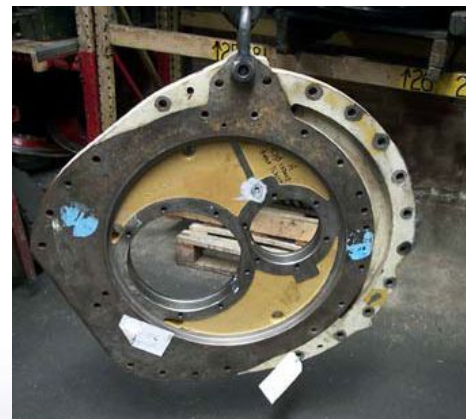
Metallise & grind bores on bevel gear assembly.
