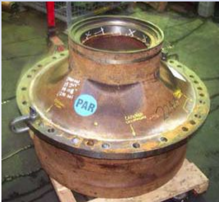
Reclaim duo cone seal areas, race bores and segment flange on D11 hub.
