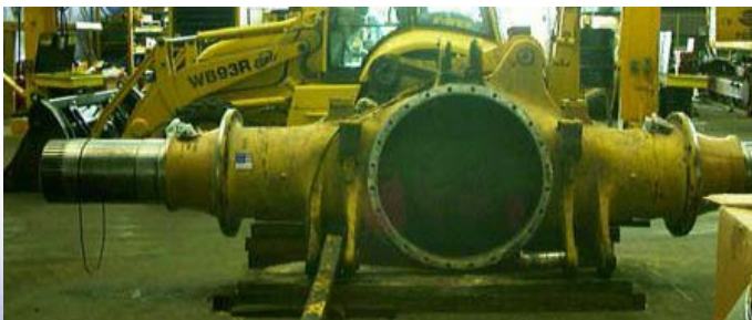
Reclaim axle journal areas on rear differential housing.
