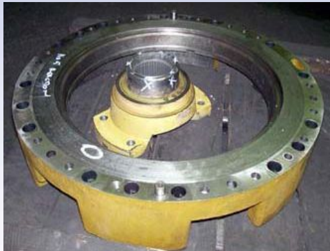
Reclaim seal bore and reaction face. Metallise and grind seal area on yoke.
