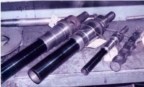
Refurbish mono pump parts.
