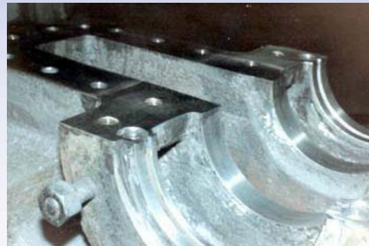
Metallise & grind ring seats on pump casings.
