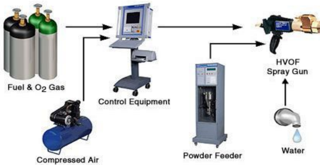
Typical Diamond Jet HVOF System
